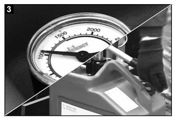
While holding the shore at the desired height, close the 1/4 turn release valve on pump can and pump the handle on the can to build pressure between 750-1500 PSI.
