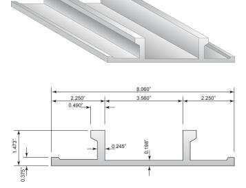
**Cross Section of Standard Vertical Rail**
