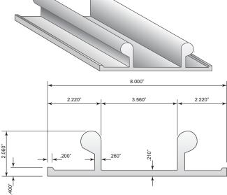
**Cross Section of Heavy-Duty Vertical Rail**
