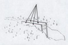
WARNING: Lift eyes are designed and intended for assembly and lifting only. Do not pull or lift by eyes when shied is stuck or has pressure against it. Loosen shield by pulling on spreader bars or digging along sides before using lift eyes.
