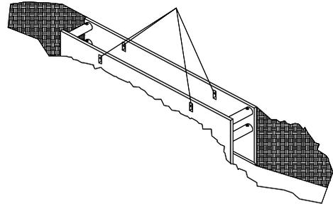
6. **WARNING:** Lift eyes are designed and intended for assembly and lifting only. Do not pull or lift by eyes when shield is stuck or has pressure against it. Loosen shield by pulling on spreader or digging along sides before using lift eyes.
