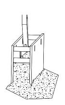
Excavate until soil begins to crumble beyond desired trench width.
