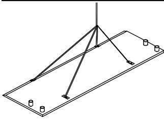
1. Remove from truck by lifting panels with 4 point lift lugs. Always use OSHA approved slings.
