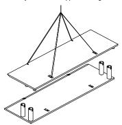
Set matching panel over bottom panel. Install Spreader pipes in collars and insert pins and keepers.
