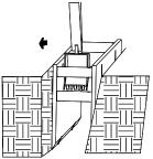
Pull shield forward by front spreaders or pulling eyes.
