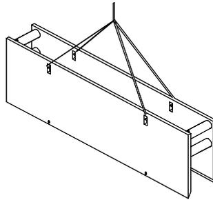
5. Place sling in top 4 lift lugs. Stand shield and install into trench.
