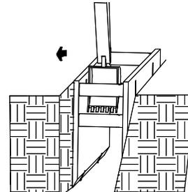
3. Pull shield forward by front spreaders or pulling eyes. Continue excavating and pull shield forward. Back fill as work progresses.
