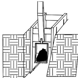
2. Perform desired work, then excavate in front of shield.
