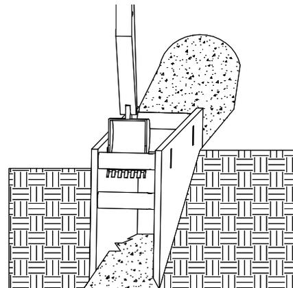
3. Perform desired work, then pull shield forward and up at appropriate angle and repeat steps (2) and (3) as necessary.
