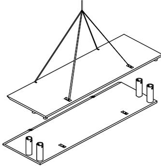
4. Set matching panel over bottom panel. Install Spreader pipes in collars and insert pins and keepers.
