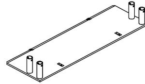
3. Set the spreader pipes over the collars and insert pins and keepers.
