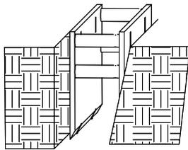
1. Excavate trench to grade, slightly wider than shield. Lift and lower shield into trench.
